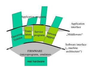
Fig. 2: The layers of a computer system
